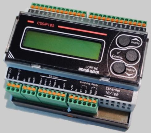
The CSSIP105 is a serial to parallel converter for a SSI encoder. The CSSIP105 retransmits on its parallel outputs (binary or gray format) the encoder value read by the SSI communication. The LCD display allows fast diagnosis of the properly functioning (input value display, physical ranges, outputs state).
